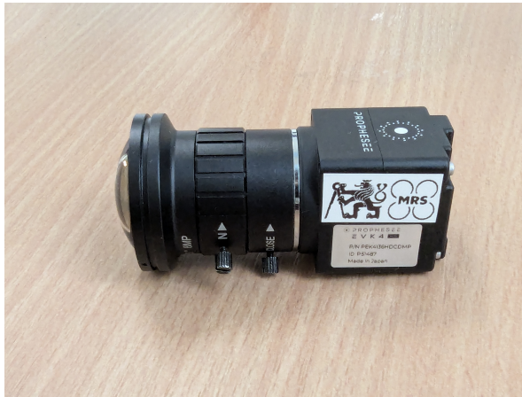
(a) The event-based camera EVK4 from Prophesee with a 2.5mm fisheye lens.
