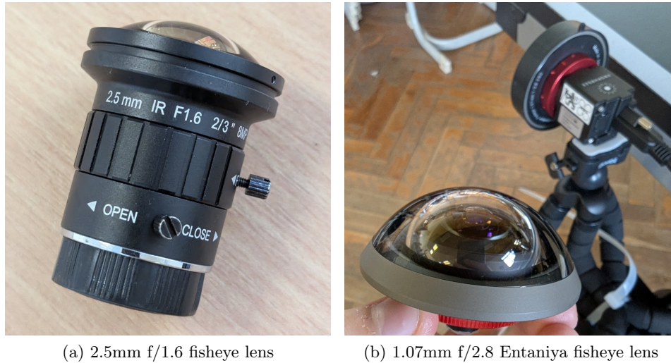
Figure 3.2: Lenses used during the calibration, a 187 degree lens in Fig. 3.2a and Entaniya 280 degree lens in Fig. 3.2b.
